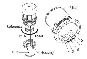
The flow rate depends on the position of the reference (located on the cartridge body) in the seat of the plastic cup.
